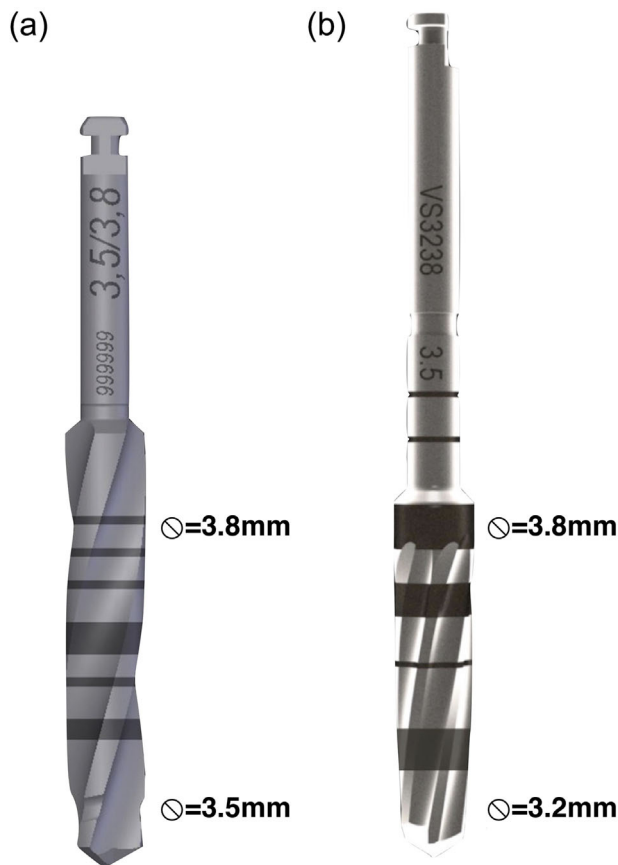
Figure 2. The CAD images of the (a) Regular (R) and (b) Versah drill, illustrating the geometric configurations.
