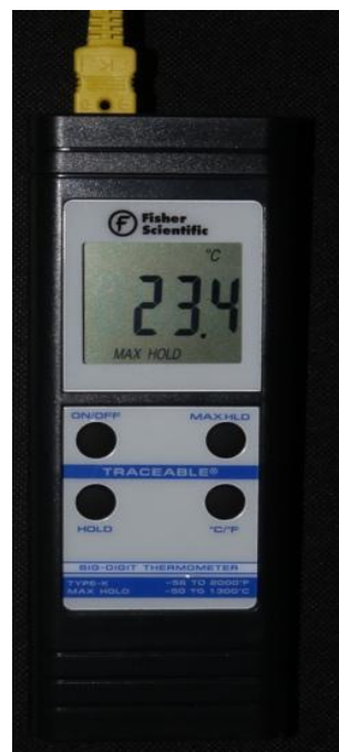
Figure 2. K-type thermocouple (Fisher Scientific 15-078-187, range -58 to 2000 °F, resolution 0.1^{\circ}/1^{\circ} , sampling rate 2.5 times per second) with an ultra-fast response naked bead probe that was used to measure the temperature.
