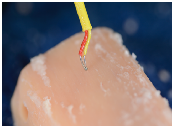
Figure 6. The initial temperature was recorded holding the K-Type thermocouple probe against the bony outer cortical layer (Step 1) [24].
