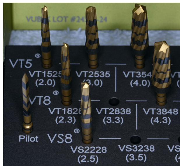
Figure 2. The bur sequence protocol (1.6, 2.0, 2.3, 2.5, 3.0, 4.0, and 4.3) used for the preparation of the osteotomies in every group, according to manufacturer's recommendations of a \varnothing 5.0 mm \times 12 mm bone level implant.
